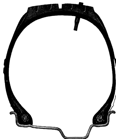
Figure 11—Sealing Plug Correctly Installed
