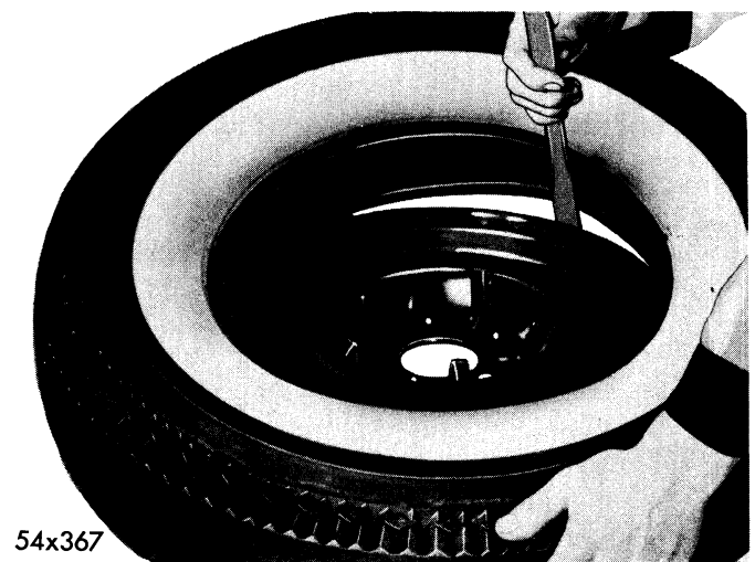
Figure 2—Installing Tire Beads
