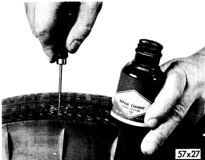
Figure 9—Lubricating Puncture with Cement
