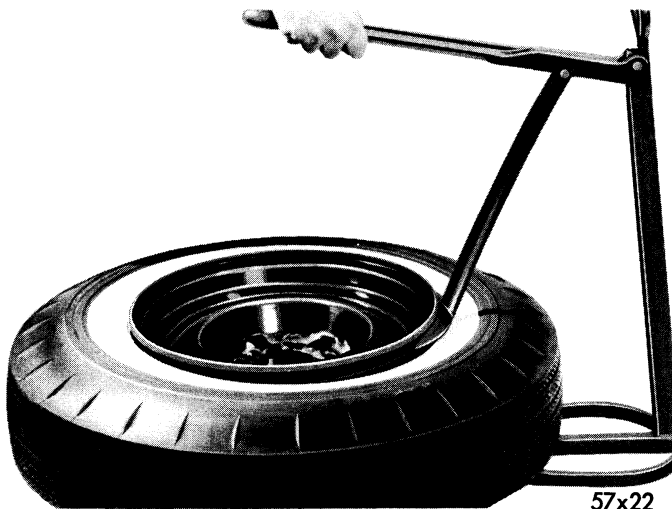
Figure 1—Removing Tire from Rim with Tool C-715
