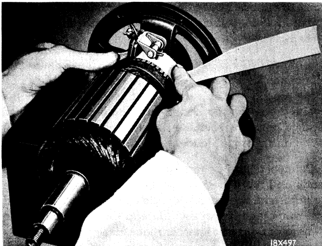
Figure 12—Seating Generator Brushes
