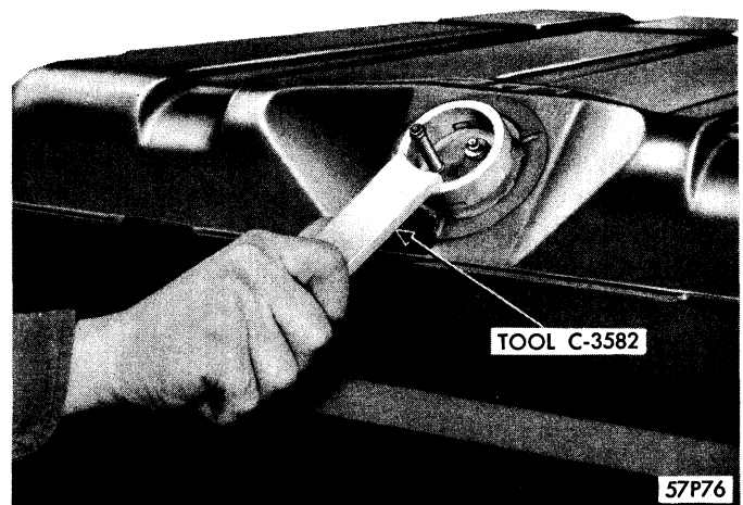
Figure 3—Removing Retainer with Tool C-3582
