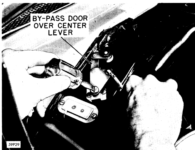
Figure 11—Adjusting by-pass door
