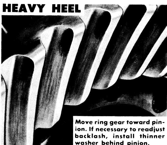
Figure 29—Gear Tooth Contact Patterns
