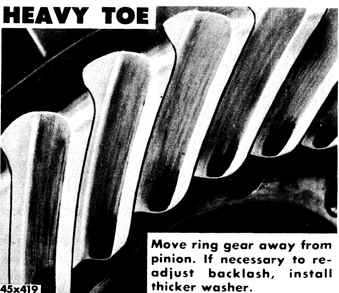
Figure 29—Gear Tooth Contact Patterns
