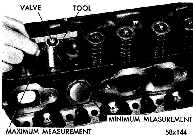
Figure 64—Checking Installed Height of Valve—
