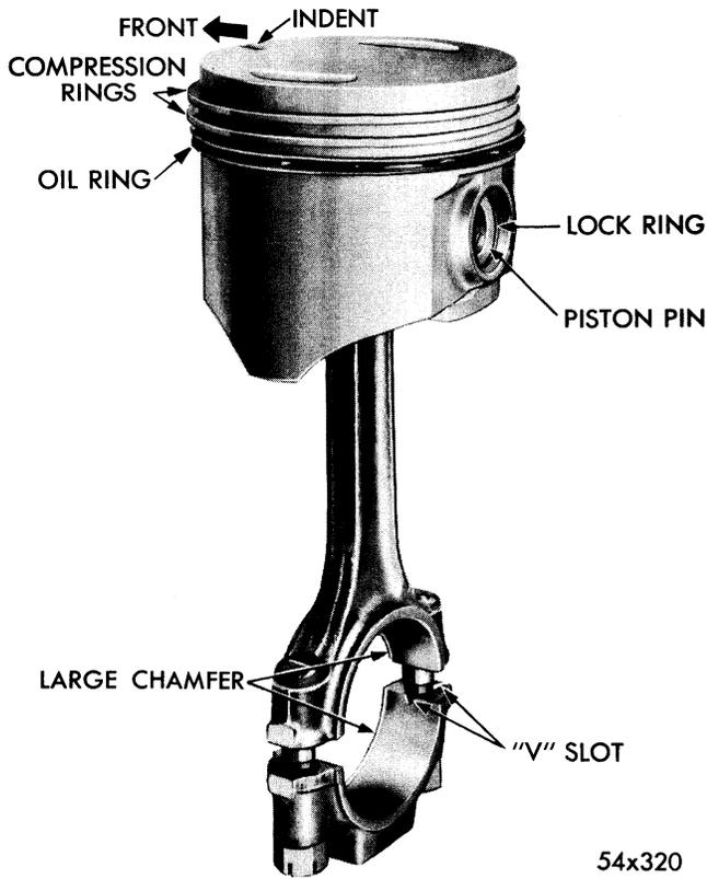
**Figure 17—Piston and Connecting Rod Assembly—
