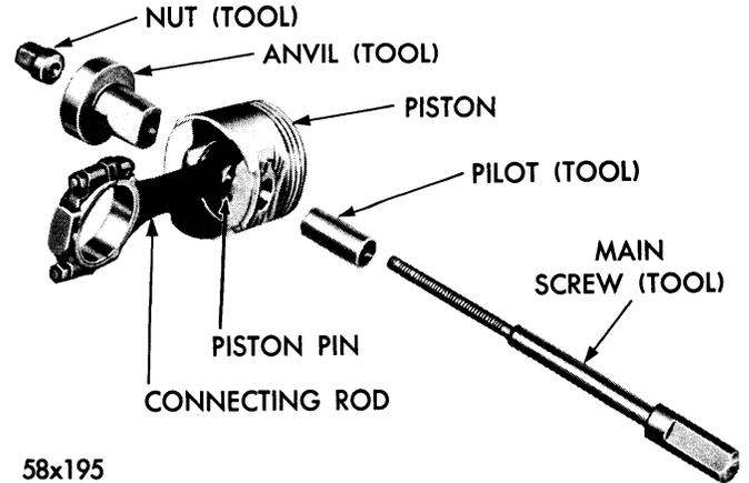
**Figure 18—Tool Arrangement for Removal of Piston
