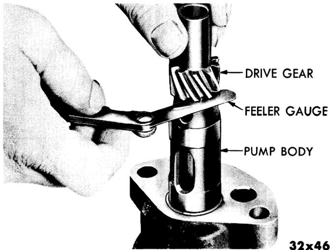
Figure 93—Measuring End Play of Oil Pump Drive Shaft—6 Cylinder Engine
