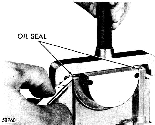
Figure 33—Trimming Rear Main Bearing Oil Seal—350 Cubic Inch V-8 Engine
