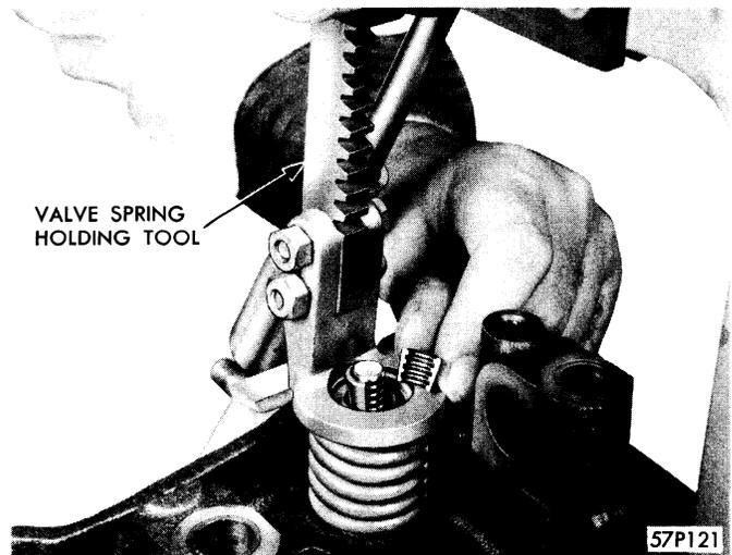
**Figure 54—Installing or Removing Valve Locks**
