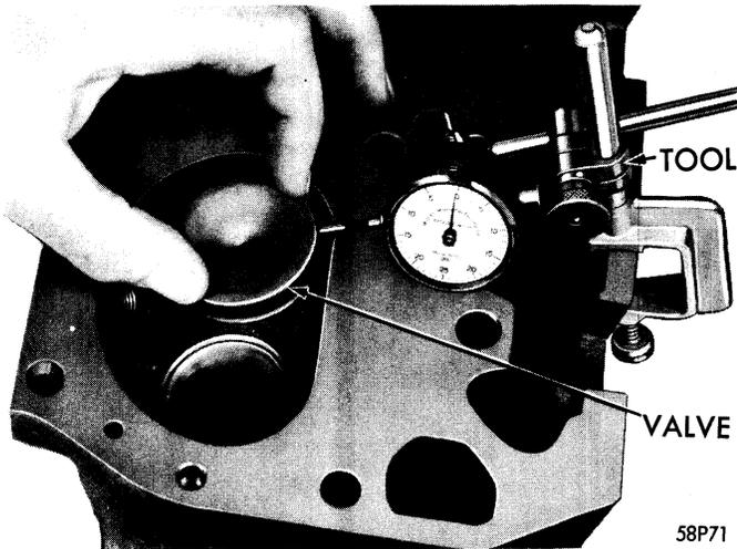
**Figure 58—Checking Valve Guide Clearance—
