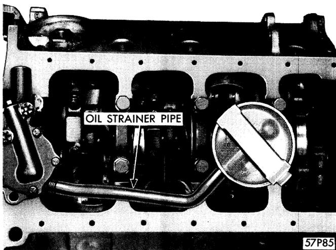
Figure 95—Oil Strainer—V-8 Engine—277, 301 and 318 Cubic Inch Engine
