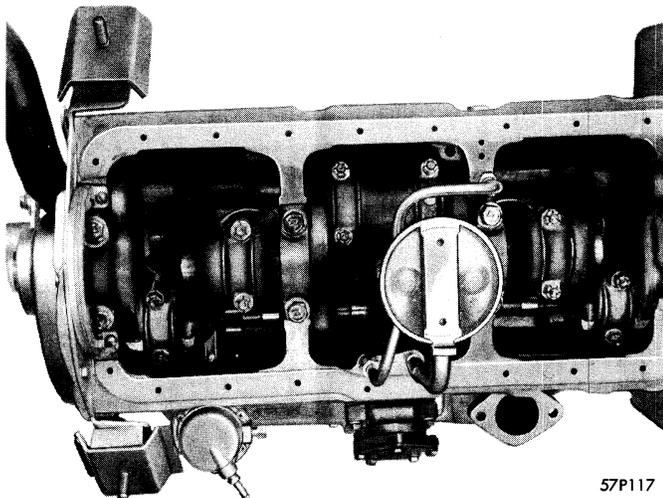
Figure 94—Oil Strainer—6 Cylinder Engine
