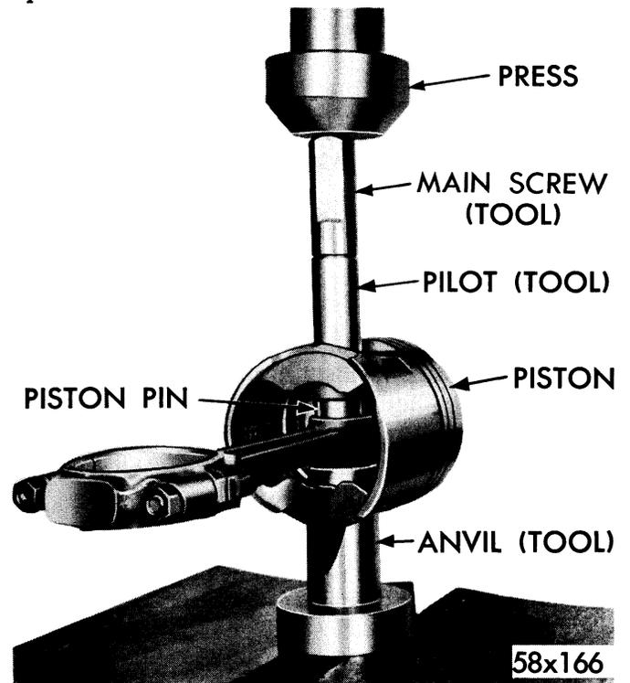
**Figure 19—Removing Piston Pin—350 Cubic Inch Engine**
