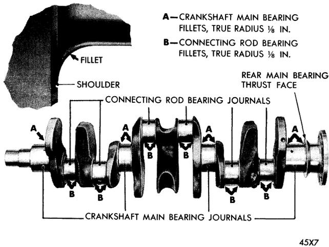
**Figure 26—Crankshaft and Connecting Rod Bearing Fillets—6 Cylinder Engine**
