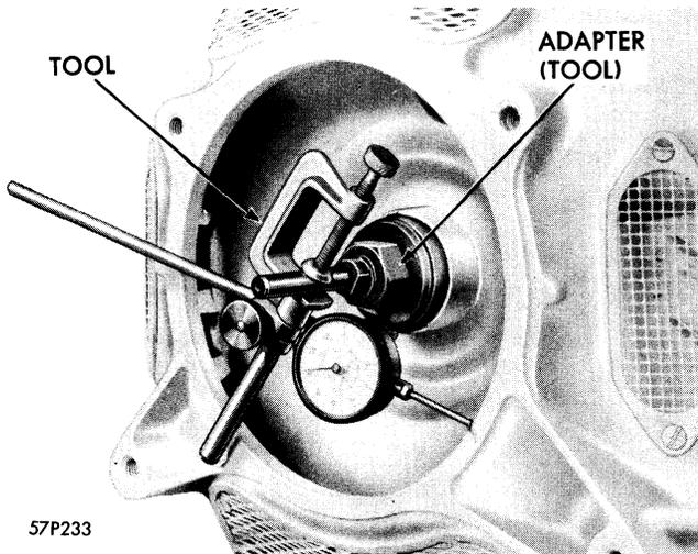
Figure 103—Checking Converter Housing Bore Runout
