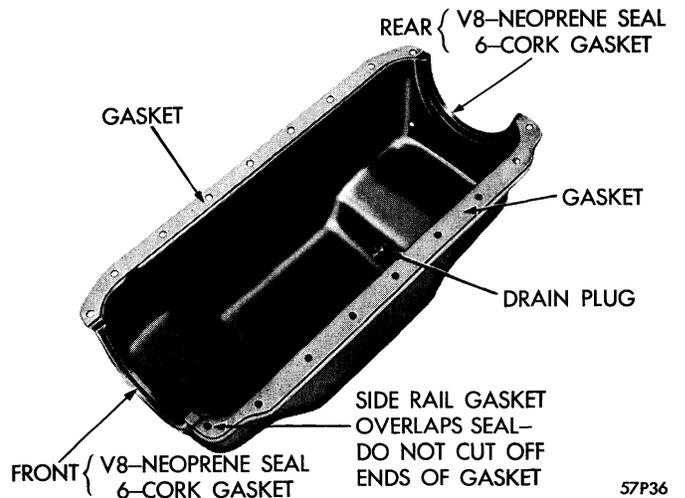
Figure 6—Oil Pan Gaskets and Seals Installed
