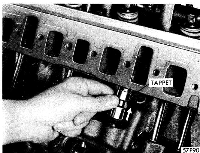
**Figure 40—Removing Mechanical Tappet—V-8 Engine**
