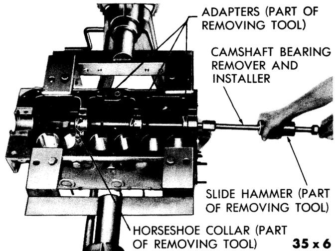
**Figure 48—Removing Camshaft Bearings—6 Cylinder Engine**
