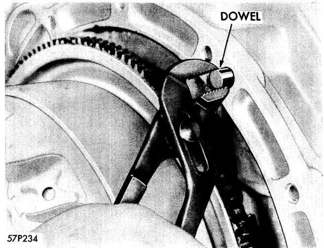
Figure 105—Removing Dowel Pin
