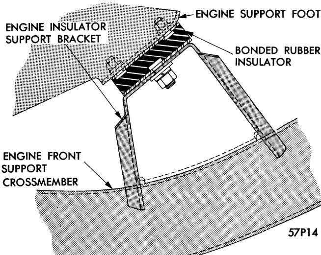
Figure 80—6 Cylinder Engine Mount—Front
