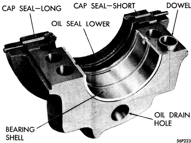
Figure 32—Rear Main Bearing Cap and Seals—277, 301 and 318 Cubic Inch V-8 Engine
