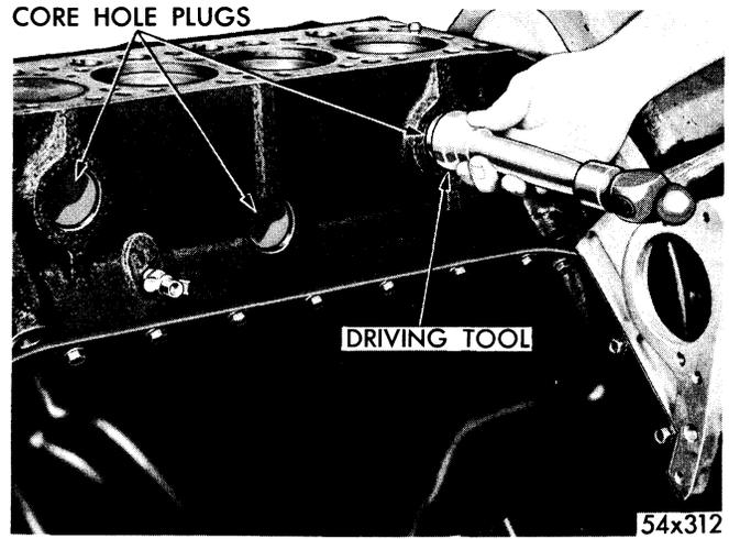
**Figure 9—Installing Cylinder Block Core Hole Plug**
