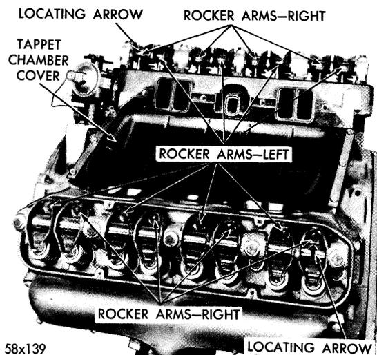
**Figure 2—Rocker Arms and Tappet Chamber Cover—350 Cubic Inch Engine**
