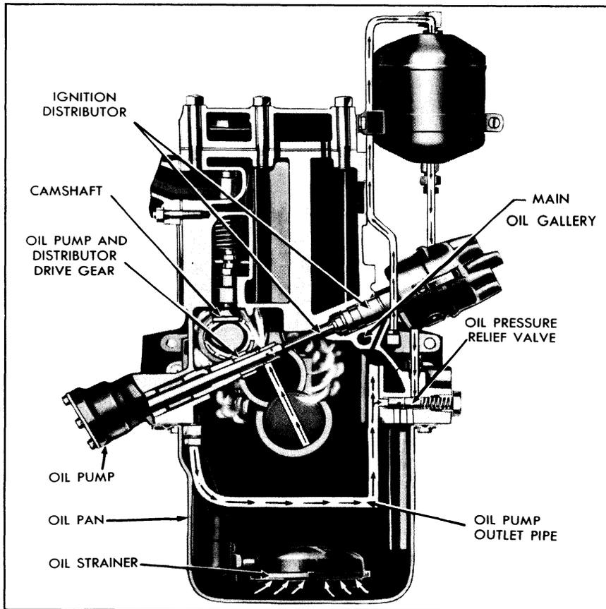
**Pressure relief valve used with by-pass type oil filter**
