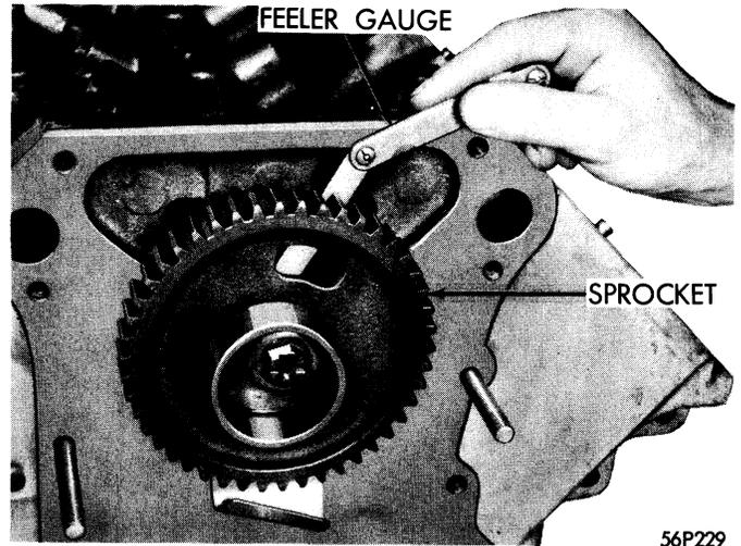
Figure 43—Measuring Camshaft End Play—V-8 Engine—277, 301 and 318 Cubic Inch Engine
