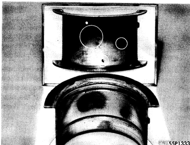
**Figure 28—Result of Dirt on Back of Bearing Insert**
