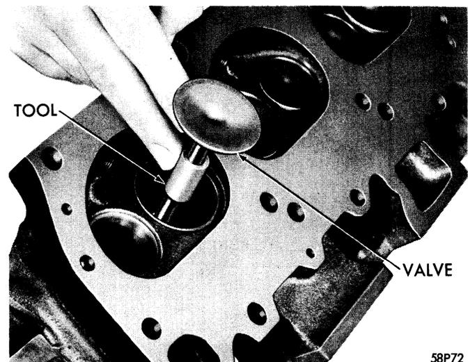
**Figure 56—Installing Valve Guide Sleeves for Checking
