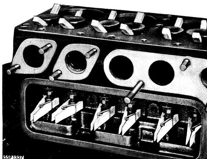
**Figure 41—Holding up Valves and Tappets for Camshaft Removal—6 Cylinder Engine**
