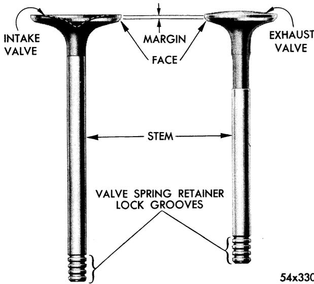
**Figure 59—Intake and Exhaust Valve Nomenclature**
