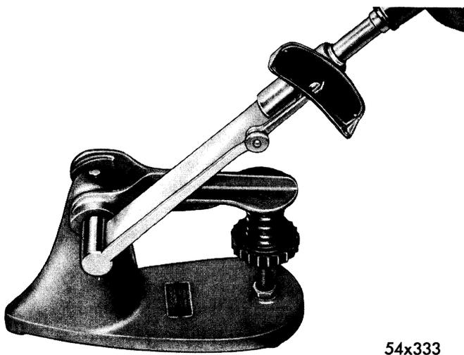
Figure 61—Testing Valve Springs
