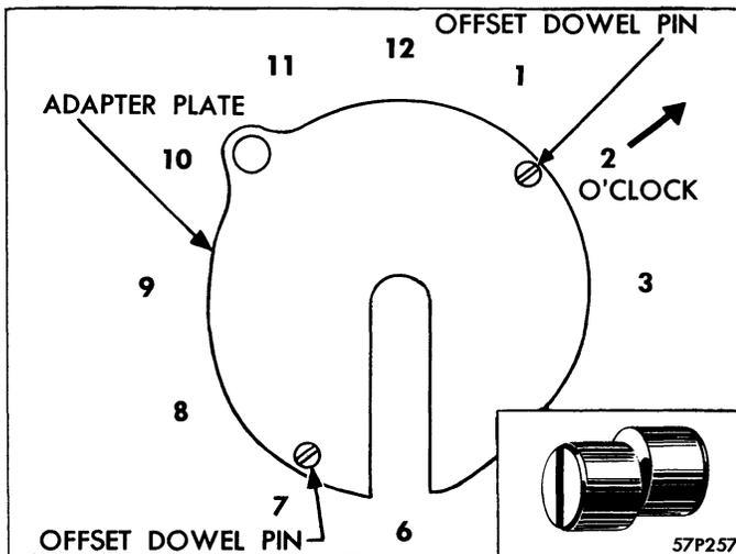
Figure 104—Adapter Plate and Inset of Offset Dowel
