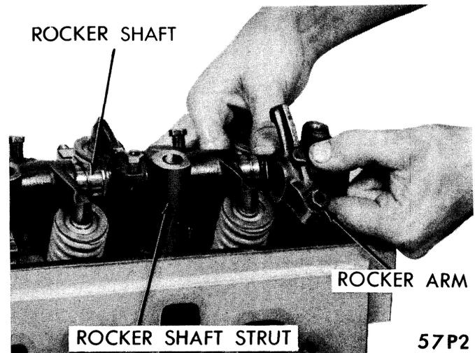
**Figure 68—Installing Rocker Arms**
