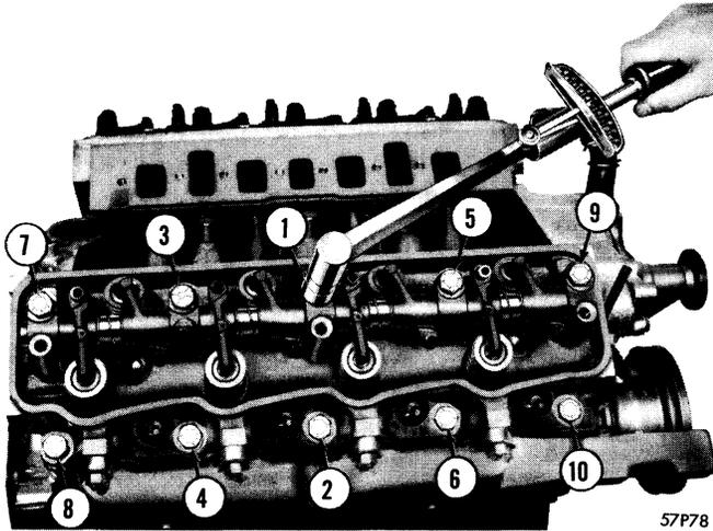
Figure 4—Sequence for Tightening Cylinder Head—V-8 Engine—277, 301 and 318 Cubic Inch Engine
