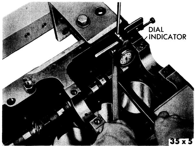
Figure 44—Measuring Camshaft Bearing Clearance—6 Cylinder Engine Typical of V-8 Engines
