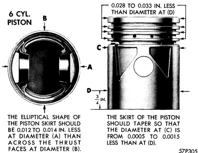
Figure 12—Piston—6 Cylinder Engine
