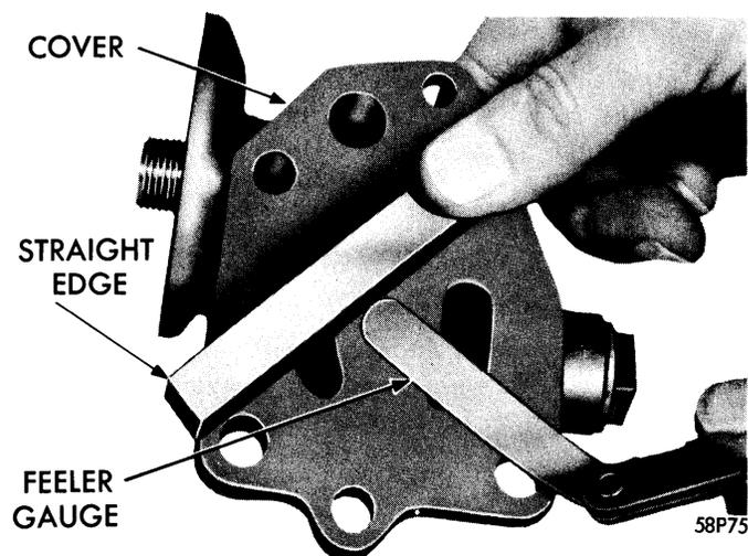
Figure 84—Checking Oil Pump Cover—
