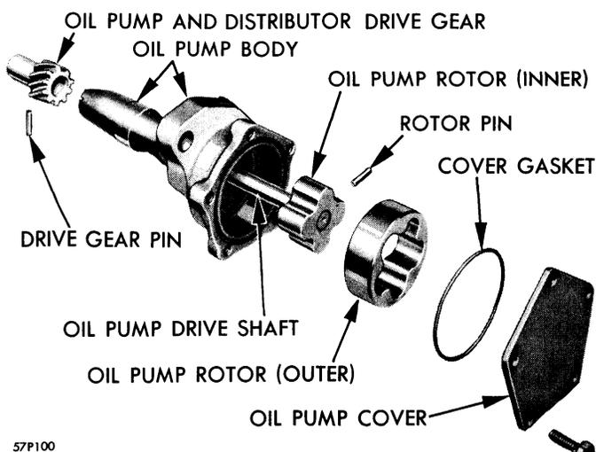
Figure 83—Oil Pump—6 Cylinder Engine
