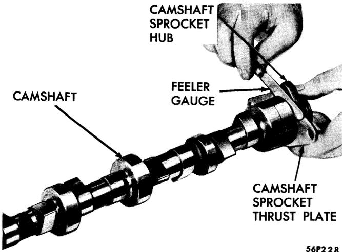
Figure 42—Measuring Camshaft End Play—6 Cylinder Engine
