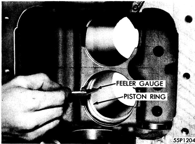
**Figure 23—Measuring Piston Ring Gap—6 Cylinder Engine**
