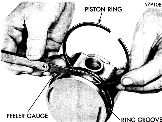
**Figure 24—Checking Piston Ring Groove Clearance**
