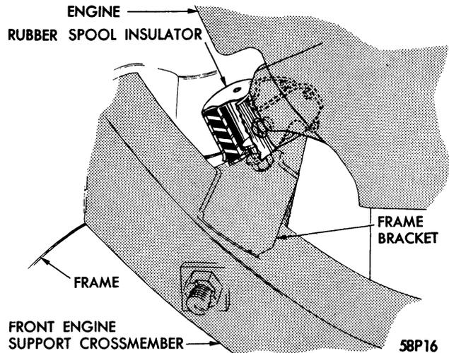
Figure 79—V-8 Engine Mount—Front
