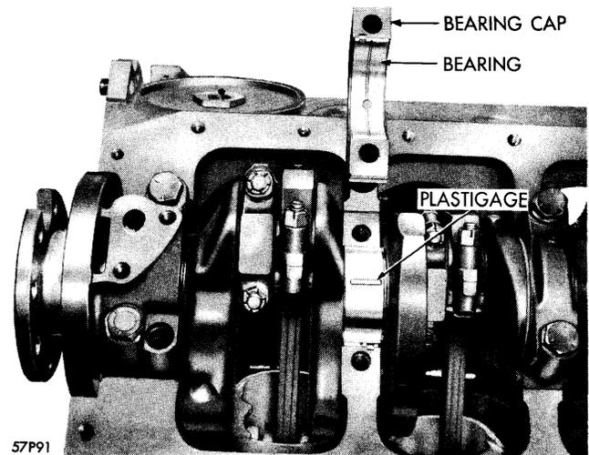
Figure 29—Checking Main Bearing Clearance with Plastigage
