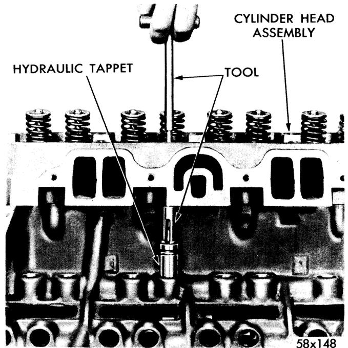
Figure 72—Removing Hydraulic Tappet—350 Cubic Inch Engine
