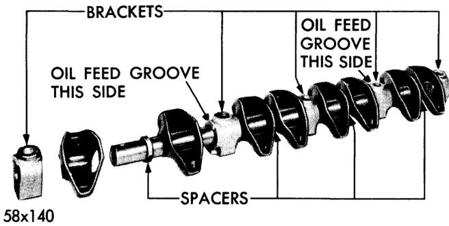
Figure 70—Rocker Shaft Assembly—350 Cubic Inch Engine
