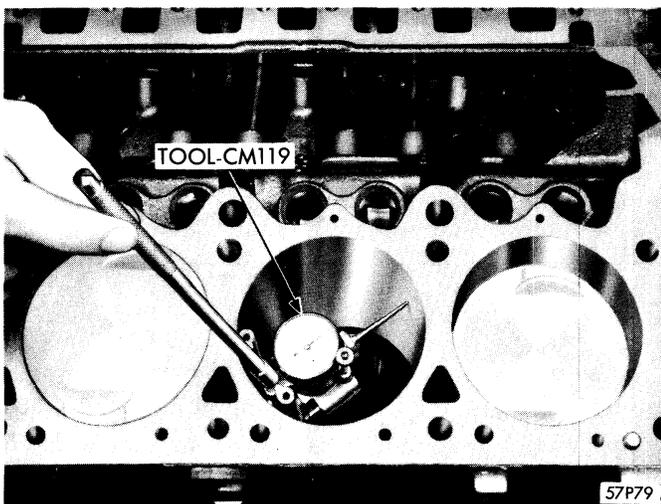
**Figure 8—Checking Cylinder Bore for Out-of-Round or Taper**
