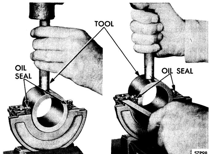
Figure 31—Installing Rear Main Bearing Oil Seal—277,
