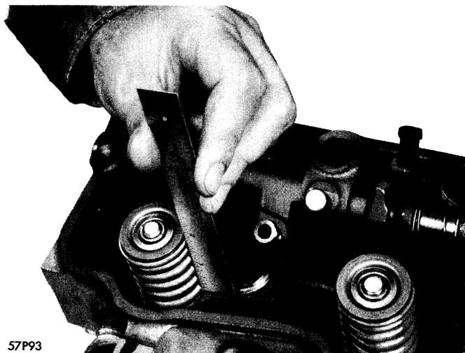
Figure 63—Checking Installed Height of Spring—
