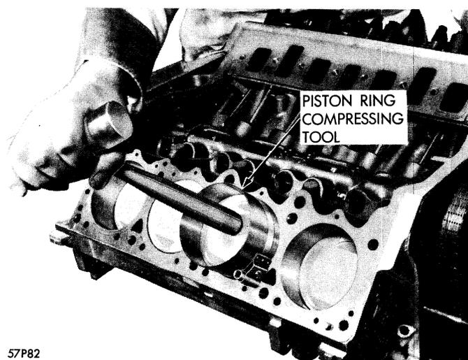
**Figure 39—Installing Piston, Ring and Connecting Rod Assembly—V-8 Engine**
