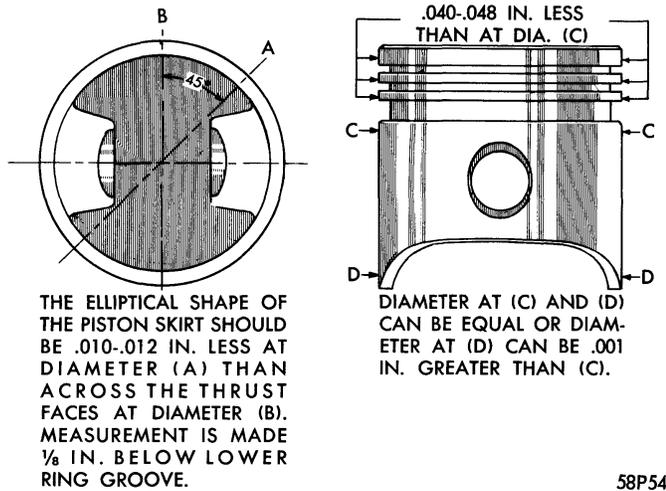
Figure 11—Piston—V-8 Engine—350 Cubic Inch Engine
