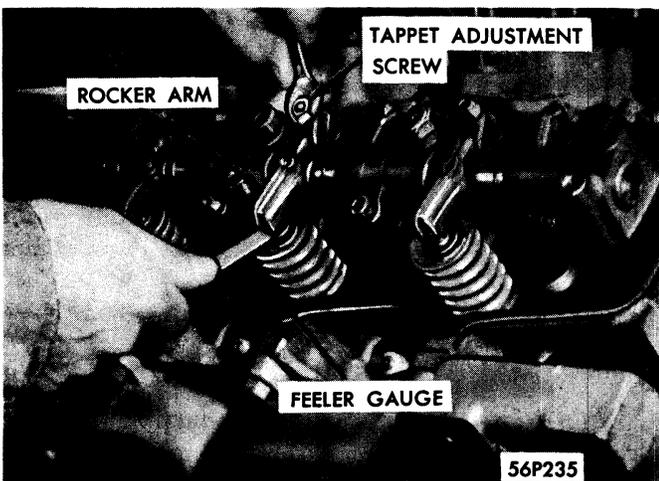
Figure 71—Adjusting Mechanical Tappets—277, 301 and 318 Cubic Inch Engine
