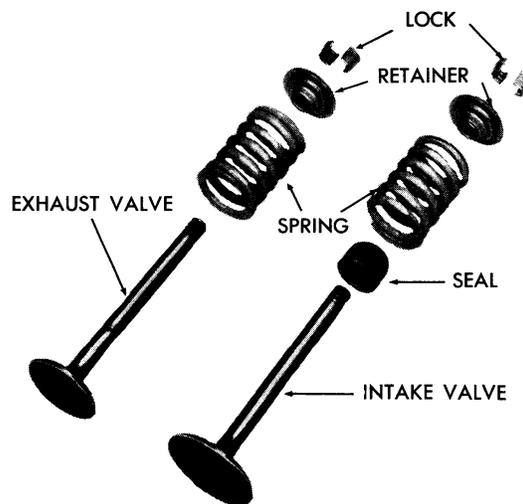
Figure 65—Intake and Exhaust Valve and Related
