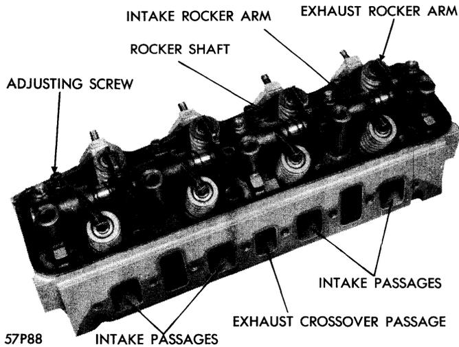
**Figure 66—Cylinder Head Assembly**
