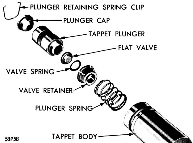
Figure 73—Hydraulic Tappet—Disassembled—350 Cubic Inch Engine
