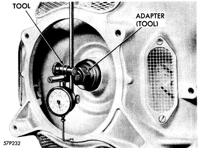
Figure 106—Checking Converter Housing Face Runout
