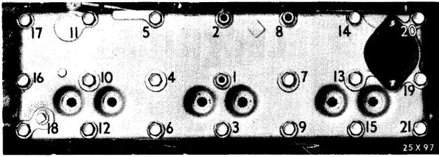
Figure 3—Sequence for Tightening Cylinder Head—6 Cylinder Engine
