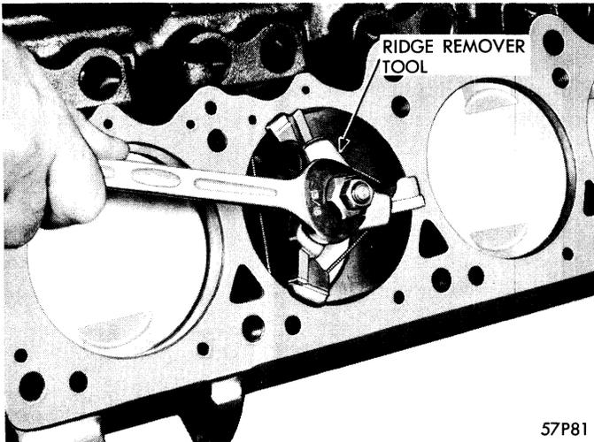
**Figure 7—Removing Cylinder Bore Ridge**
