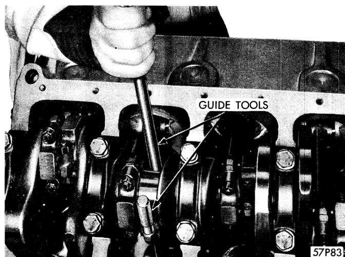
**Figure 38—Guiding Connecting Rod on Crankshaft Journal—V-8 Engine**
