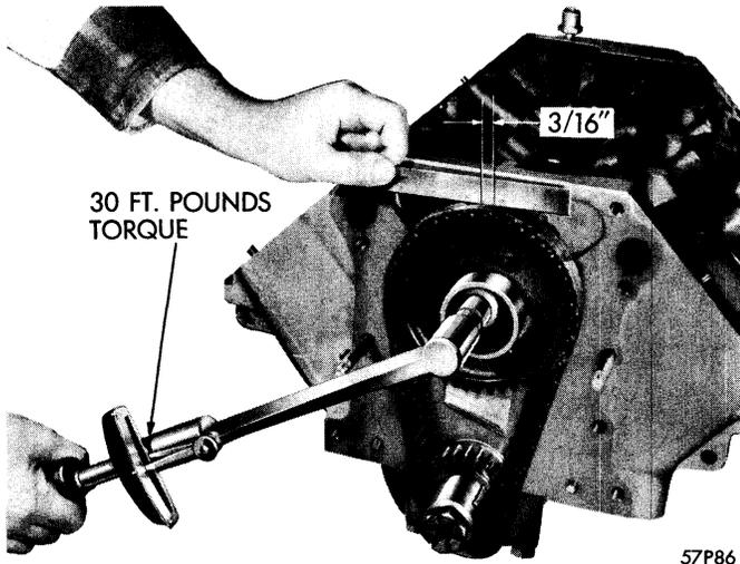
**Figure 53—Measuring Timing Chain Stretch—
