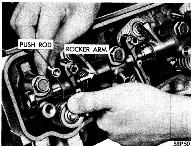
**Figure 1—Removing Push Rods from V-8 Engine—277, 301 and 318 Cubic Inch Engine**
