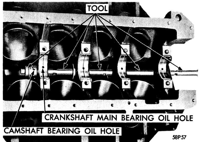
Figure 45—Installing Camshaft Bearings—350 Cubic Inch V-8 Engine Typical of 277, 301 and 318 Cubic Inch Engine
