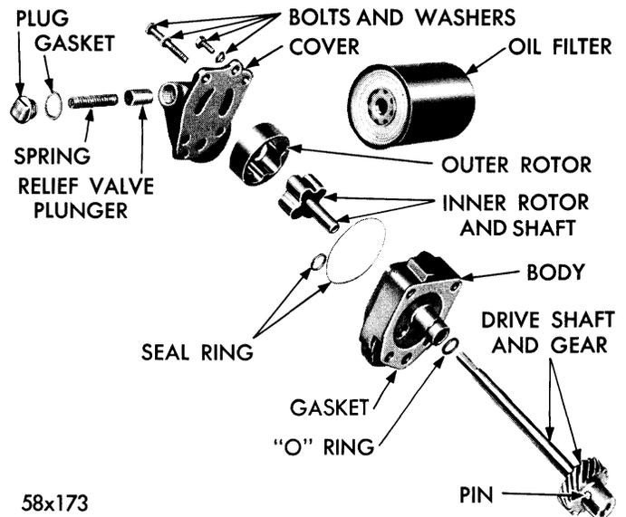
Figure 82—Oil Pump—V-8 Engine—
