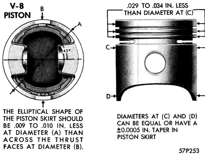
Figure 10—Piston—V-8 Engine—277, 301 and 318 Cubic Inch Engine
