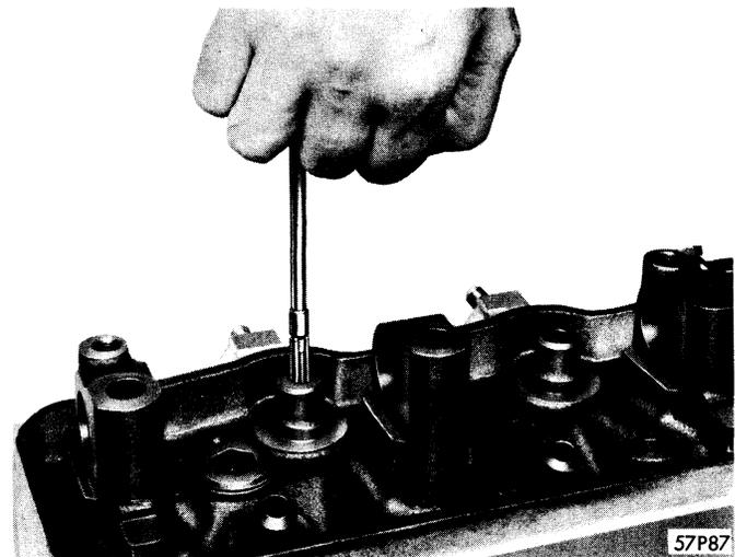
**Figure 55—Cleaning Valve Guide—277, 301 and
