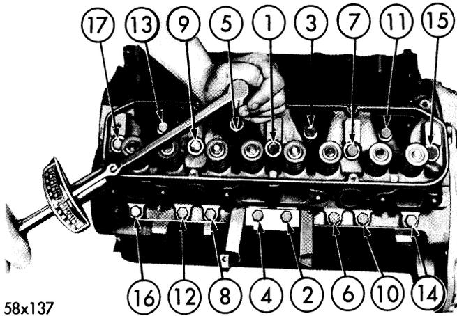
Figure 5—Sequence for Tightening Cylinder Head—V-8 Engine—350 Cubic Inch Engine
