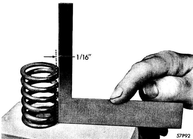
Figure 62—Checking Trueness of Valve Springs
