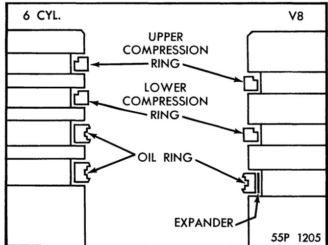
**Figure 25—Piston Rings Assembled to Piston**
