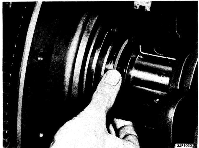
Figure 35—Installing Upper Seal—6 Cylinder Engine
