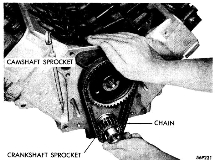
**Figure 52—Installing Timing Chain, Sprocket and
