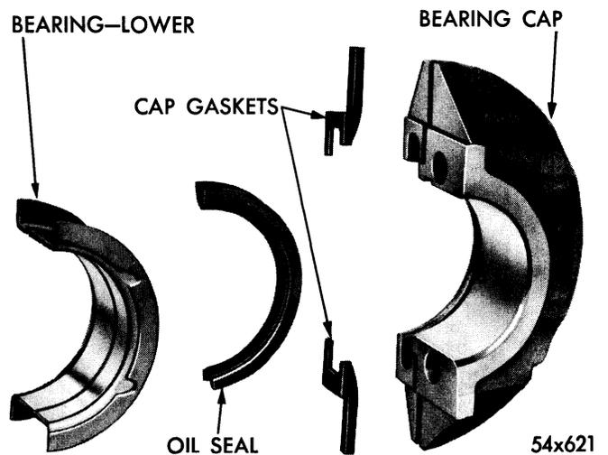
Figure 34—Rear Main Bearing and Cap Seals—6 Cylinder Engine
