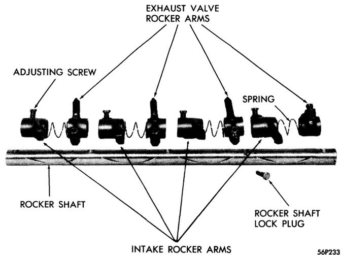
**Figure 67—Rocker Shaft Assembly**
