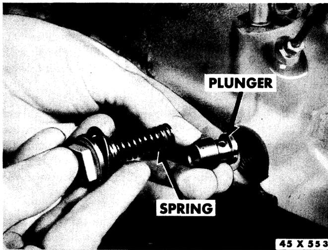
Figure 96—Oil Pressure Relief Valve—6 Cylinder Engine
