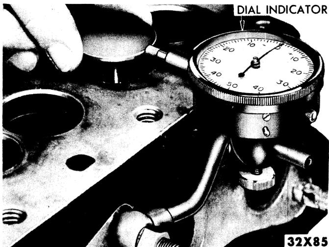
Figure 75—Measuring Valve Stem to Guide Clearance
