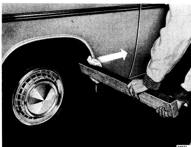
Figure 39—Closing Gap Between Fender and Sill Panel
