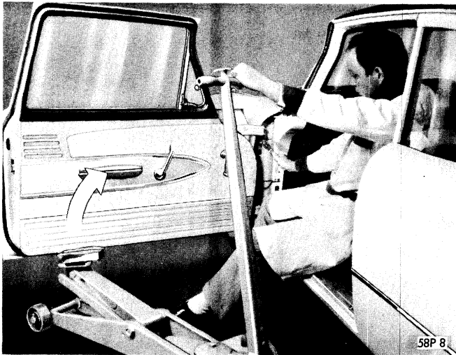
Figure 60—Moving Upper Half of Door In Toward Pillar
