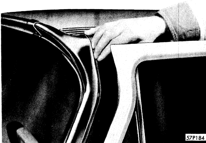
Figure 61—Leading Edge of Upper Half of Door Flange Rubs on Pillar
