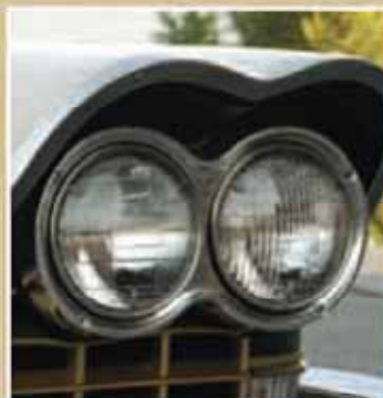
By 1959, quad/dual headlamps were pretty much an industry standard. Plymouth used that format to maximum advantage, styling the '59 front fenders to give the appearance of separate "eyebrows" for each eye.
