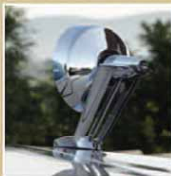
Ineffective as they were, mounted so far forward on the front fenders, even Chrysler's sideview mirrors reflected the Forward Look philosophy. Driver-side adjustment was usually remote, with manually adjustable passenger mirrors.
