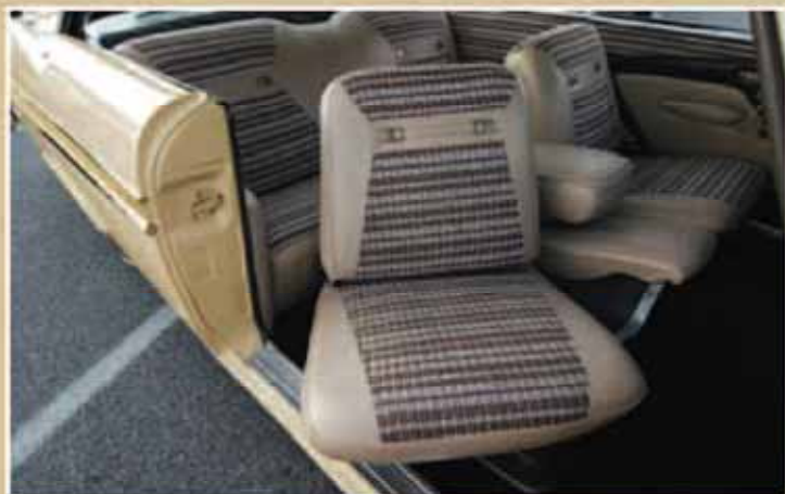
Fifties Chrysler products offered swivel front seats for easier entry and exit. They disappeared, no doubt as a cost consideration. But in 1959, they were standard on Sport Fury convertibles and hardtops.
