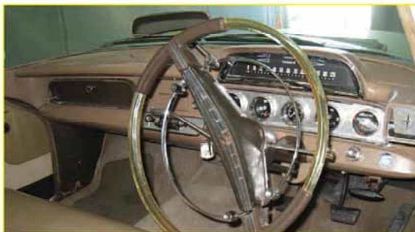
The long speedometer: All Chrysler-built full-sized cars with right-hand-drive, used '58 Dodge dashes. Note the pushbutton delete plate to the right.
