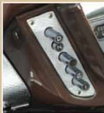
No mere two-speed PowerFlite here—an upscale transmission for an upscale car made the three-speed TorqueFlite standard in Golden Commando applications. Note the driver-side rearview mirror adjusting knob at lower left of dash.
